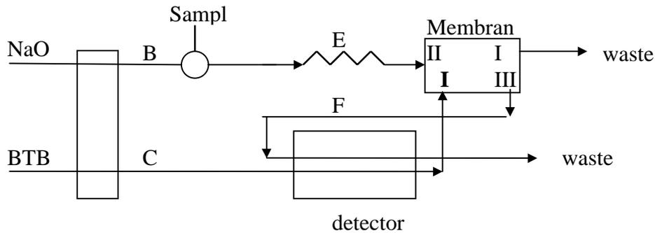
Figure 1: A schematic diagram of the Flow Injection/Gas Diffusion apparatus used for the determination of TVB-N.
