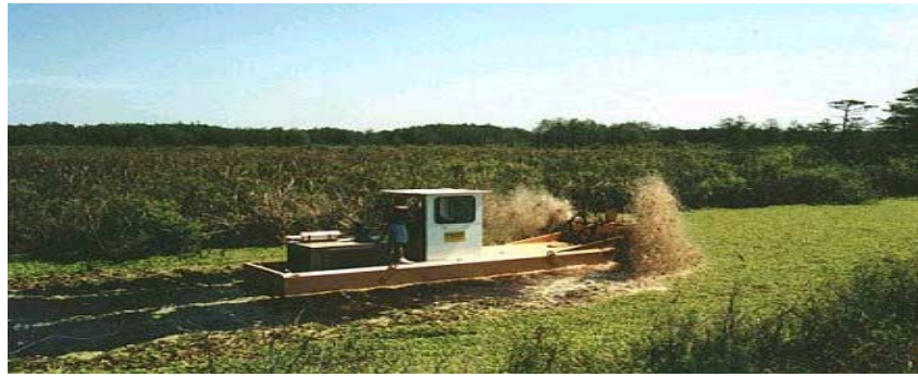
Figure 5: A Picture showing mechanical shredding of water hyacinth in Winam Gulf, Lake Victoria (Aquarius Systems 2001).
