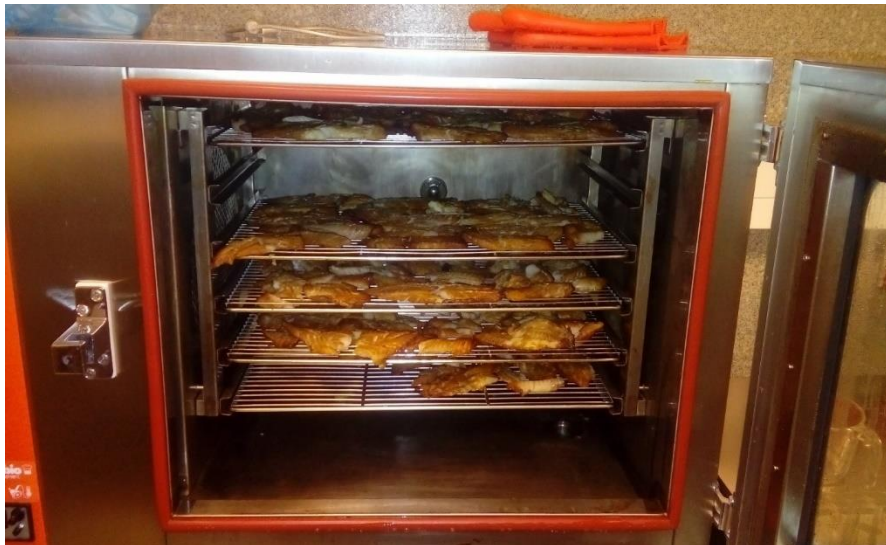
Figure 25: Fillets in drying Oven.
