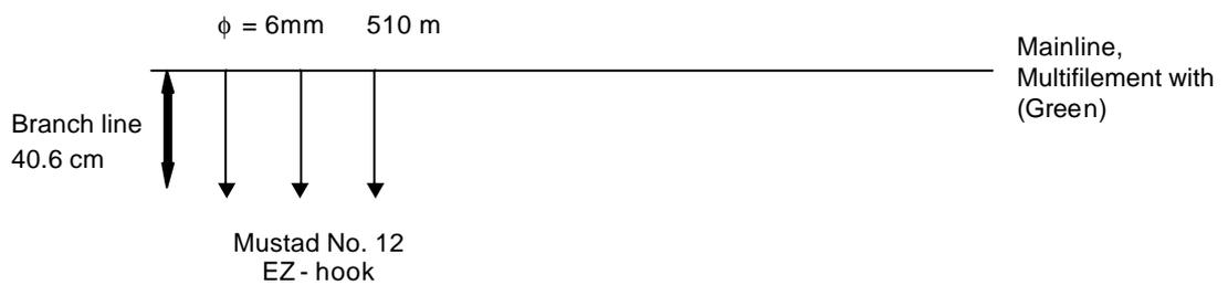
Figure 6: Gear parameters with the experimental longline gear module.
